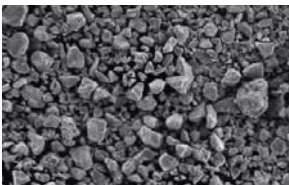
Before Plasma Spheroidization
